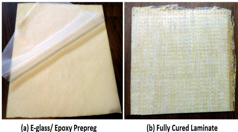
Fig. 4.1. Prepreg material and fully cured laminate
