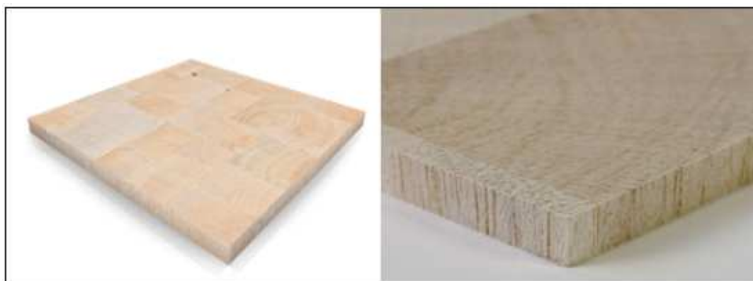
Fig. 4.2. End-grain balsa wood
